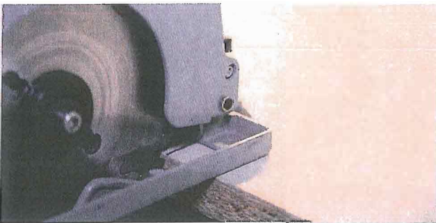
Picture No. 3: Cutting handheld circular saw.
